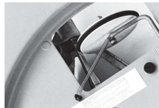
Sliding idler wheel on the conical motor shaft
