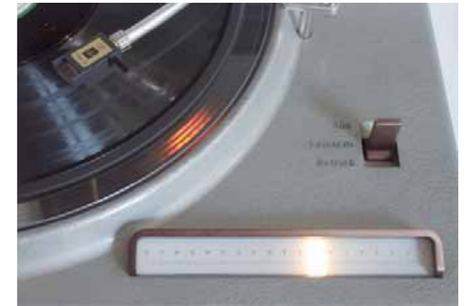
Illuminated stroboscope and display for tonearm position
